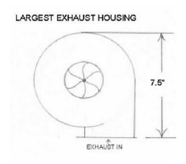
7.Exhaust must discharge vertically upward above highest point of tractor, exception of roll bars, and be securely attached. Exhaust must be at least 18: above the hood an no curved pipes or rain caps allowed. Exhaust pipe must be cross-bolted with two 3/8: grade five bolts with 1: of each other in vertical pipe and two 5/16: bolts within one inch of exhaust housing.
